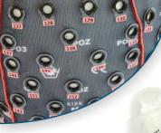
Electrode holder rings with channel labels attached to g.GAMMAcap²
